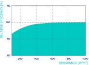
Typical module performance under low irradiance conditions in comparison to STC conditions (25  $^{\circ}$ C, 1000 W/m²).
