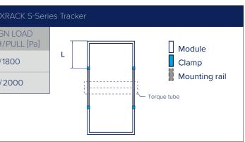
Distance between outer edge of module and middle of the clamp.
