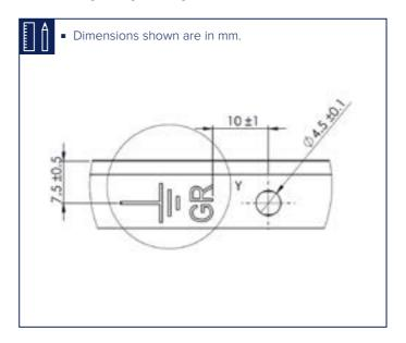
Grounding or bonding should be carried out with Zn-based coated connecting elements to avoid the galvanic coupling effect.
